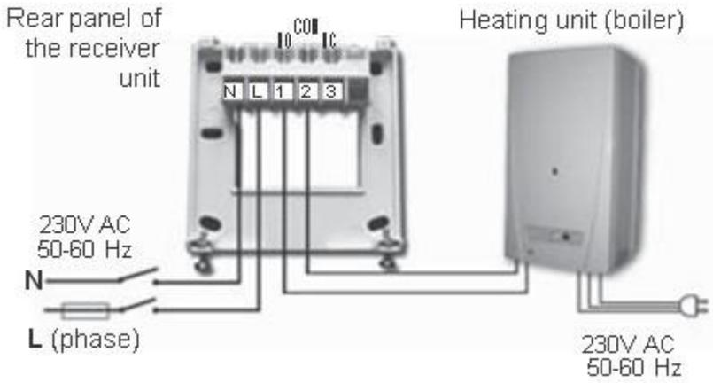
The receiver unit controls the boiler or air conditioner through a potential-free alternating relay whose connection points are: **1 (NO)**, **2 (COM)** and **3 (NC)**. Connect the two connection points of the heating or cooling equipment to be controlled to terminals **No. 1 (NO)** and **No. 2 (COM)**, i.e. to the normally open terminals of the relay.
